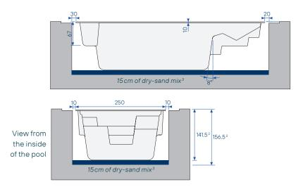
Note: the digging sizes do not take into account the necessary space for the coping stones.
